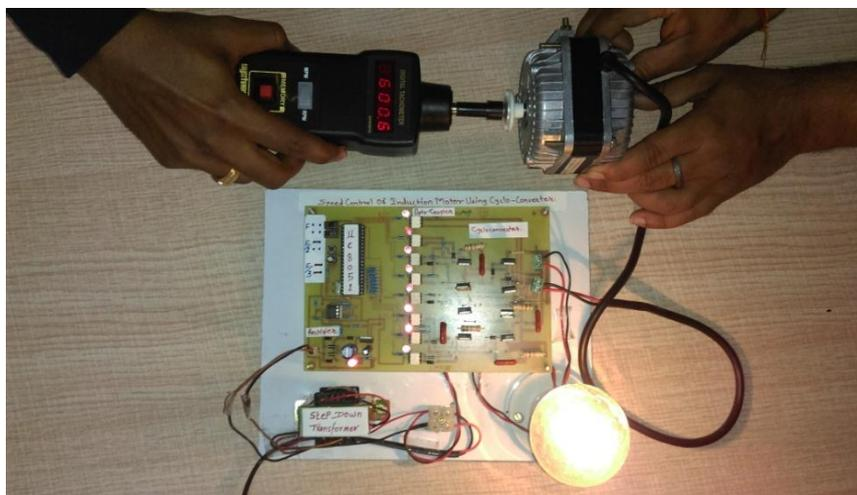
Fig. Speed of induction motor at F/2
