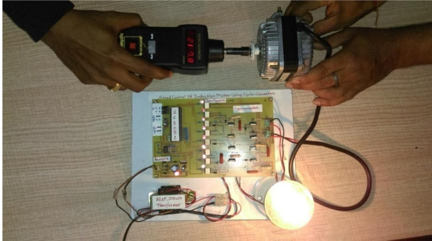
Fig. Speed of induction motor at F/3
