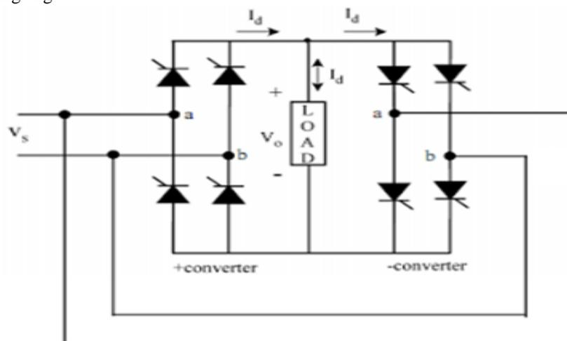
**Fig. 1:** single-phase to single-phase Cyclo-converter with mid-tap transformer
